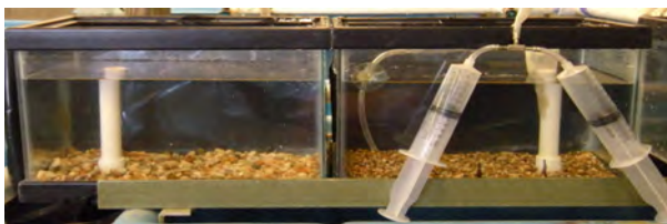
Fig. 1: Experimental set-up. The tank housing the test fish ( Etheostoma fonticola ) is shown with syringes and airline tubing for chemical stimulus introduction (right) and the tank housing the predator species for treatments involving visual cues (left).
