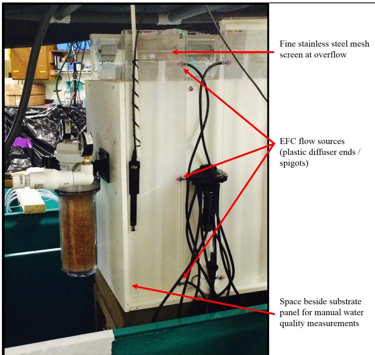
Figure 3. Photograph of RBASS environmental flow chamber design showing flow spigots and mesh screen at chamber overflow point.
