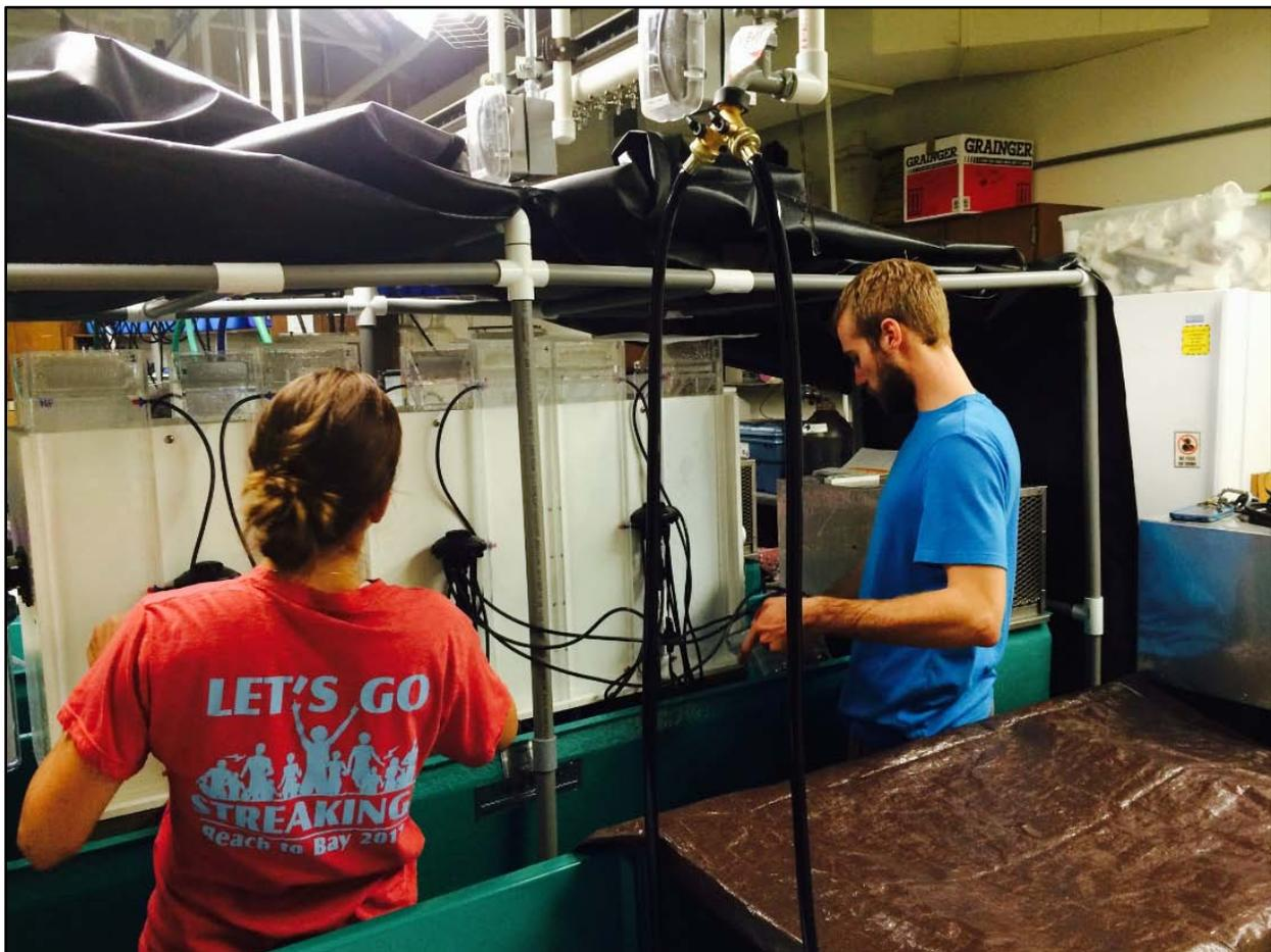
Figure 2. Photograph of RBASS system setup at the at Texas State University Freeman Aquatic Building laboratory showing six RBASS environmental flow Chambers, upwelling flow spigots, and black nylon cover.
