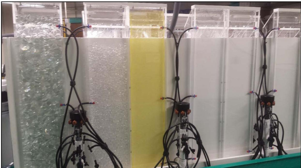
Figure 5. Photograph of RBASS system showing environmental flow chambers with different substrates tested in the *Microcylloepus pusillus* Substrate Pilot Studies.
