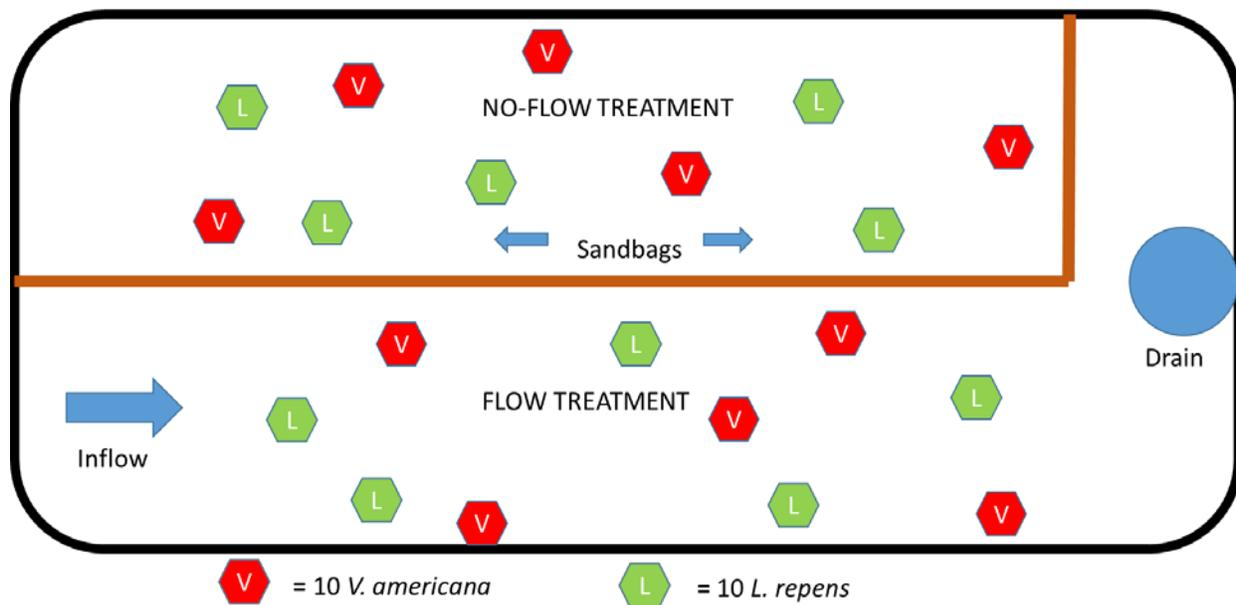
**Figure 3.** Representation of the experimental scheme for the low-flow threshold evaluation of native aquatic vegetation pond experiment. The experimental pond will be divided by a sandbag barrier, leaving approximately one half of the pond with flow-through conditions. The remaining pond area will provide conditions representative of those expected from a loss of flow in the Comal system.
